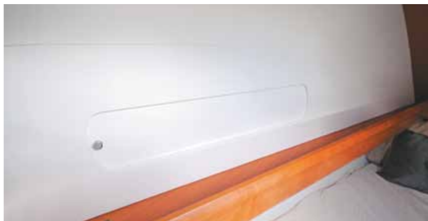
Aft cabins (above left) in three-cabin layouts have double berths and wardrobes. Saloon head (left) has a separate shower stall. In forward and aft cabins, hull ports (above photos) are covered by sliding shutters that disappear into recesses when not in use.
