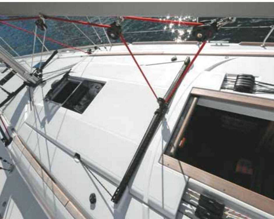
The upside of mid-boom sheeting (above) is shorter mainsheet length meaning less line to handle on gybes.
