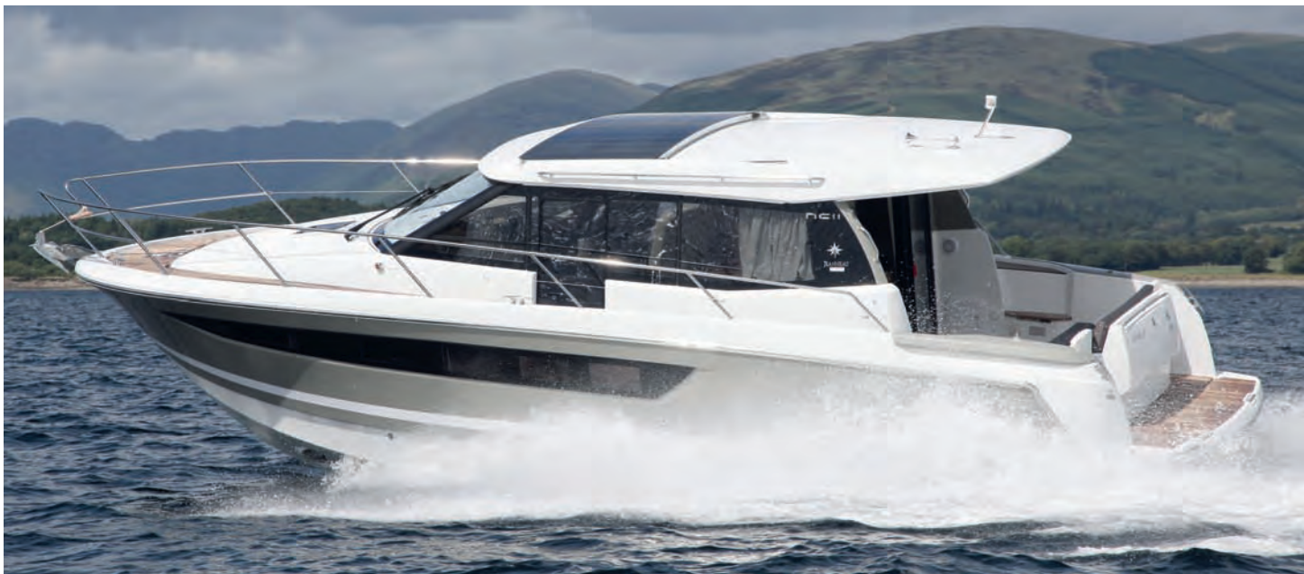
The superstructure's generous overhang does an excellent job of protecting the huge opening exposed by the four-part sliding doors
