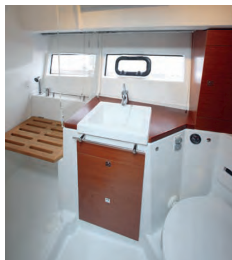
The shower is partitioned off and has its own seat
