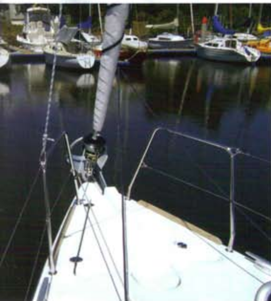
The test boat had a Manson Supreme anchor and a 1000W Muir windlass.
