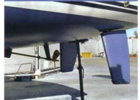
Close up showing the twin rudders and their "shoes".
