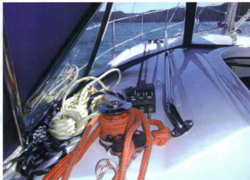
The main halyard, furling line and two reefing lines come back to a winch and a clutch of jammers on the port side of the cabin top.
